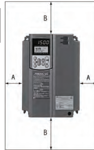
Figure 2.1-1 Mounting Direction and Required Clearances
